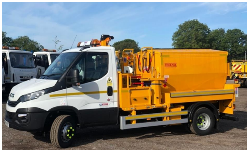
Hot-Box Pothole Repair Vehicle.
